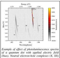
of a quantum dot with applied electric field (bias). Neutral electron-hole complexes (X, XX)as well as ones with extra hole (X+) and extra electrons (X-, X--) are visible at different biases due to the charge transfer to / from a 2DEG.
