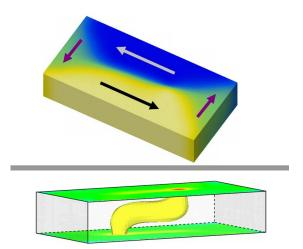
*FIG. 1:* Top: Simulatied static magnetization structure in a  $400 \times 200 \times 80$  nm<sup>3</sup> Permalloy prism. The structure is divided into four domains. On the surface, the magnetization circulates around a point (vortex). Bottom: The vortex contains a core that is stretched along the sample. The yellow surface displays the core region, where the perpendicular magnetization component exceeds a value of 70%.
