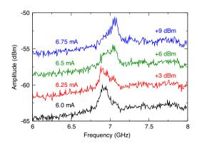
FIG. 2: Microwave spectra recorded at 5 K and in a weak field of 5 mT. All curves are taken at DC currents corresponding to the  $90^{\circ}$ -state [red area in Fig. 1(c)].
