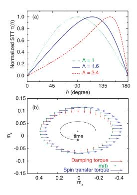
FIG. 3: (a) Angular dependence of the STT amplitude  $g(\vartheta) \sin(\vartheta)$  according to Eq. (2) for different  $\Lambda$ . (b) Representation of the STT (blue arrows) and damping torque (red arrows, enlarged by factor 5 relative to the STT) for the low-field precession in the 90°-state.
