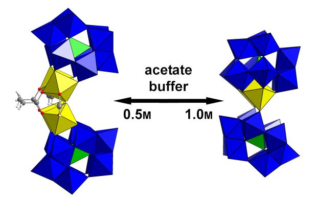
FIG. 1: Schematic metalation/demetalation reactions in aqueous solution originating from  $\{\gamma$ -Fe<sub>2</sub> $W_{10}$ Si} Keggin-based structures. The concentration of acetate surprisingly represents one critical reaction parameter. W: blue, Fe: yellow, Si: green polyhedra, acetate as ball-and-stick.
