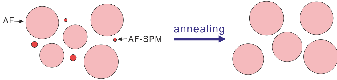
Figure 77: As-prepared MnO powder sample composed of particles with a large size distribution. Large particles with a size of \sim \mu\text{m} show AF behaviour and small particles ( \sim several hundred nm size) show AF-SPM behaviour. After annealing, particles with similar sizes ( \sim \mu\text{m} ) can be fabricated.
