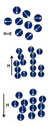
Figure 2.8.: Effect of the external magnetic field on the arrangements of the dipoles.
