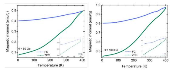
Figure 6.3.: Magnetization-temperature curves recorded in FC and ZFC modes for cobalt ferrite nanopowder in an external magnetic field of 50 Oe (left) and 100 Oe (right).
