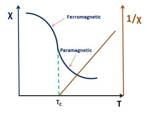
Figure 2.4.: Magnetic susceptibility vs. temperature for ferromagnetic system.
