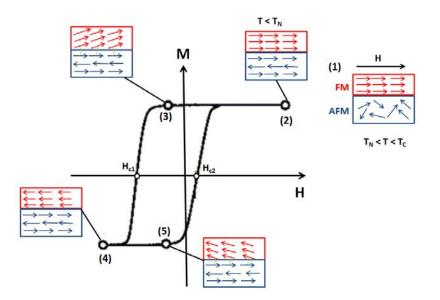
Figure 2.7.: Phenomenological picture of exchange bias for an AF-FM bilayer and illustration of the spin order during the hysteresis measurement. Inspired from [34]
