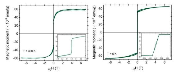
Figure 6.2.: Magnetization hysteresis curves for cobalt iron nanopowder at 300 K (left) and 5K (right).
