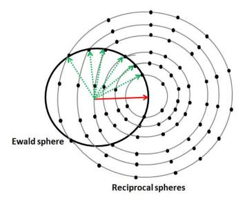
Figure 2.13.: Ewald sphere construction for powder samples.
