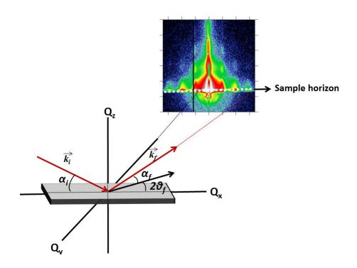
Figure 2.16.: GISAXS geometry with the reciprocal axes.
