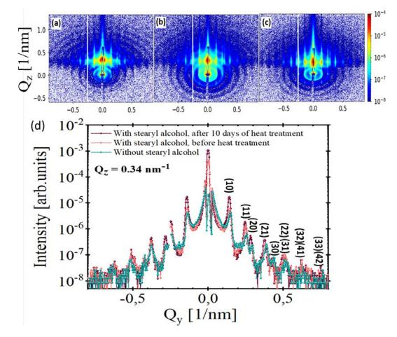
Figure 5.15.: GISAXS pattern of a monolayer of SiO<sub>2</sub> NPs deposited on silicon substrates (a) before using stearyl alcohol (b) after using stearyl alcohol, before heat treatment and (c) after 10 days heat treatment. (d) Linecuts from (a), (b) and (c) along  $Q_y$  at a constant  $Q_z = 0.34nm^{-1}$ . The Bragg peaks are indexed by assuming a 2-D hexagonal lattice with a lattice constant  $a = 51.6 \pm 0.4$  nm.
