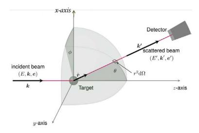
Figure 2.10.: Geometry of the scattering cross section: number of particle N per unit time dt measured by a detector at a distance r, scattered into an element of solid angle  $d\Omega$  in direction  $(\theta, \Phi)$ . Adapted from[54]
