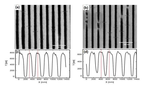
Figure 4.13.: (a) SEM image for S1\_01, (b) SEM image for S1\_02, (c) Line profile for S1\_01 and (d) Line profile for S1\_02.
