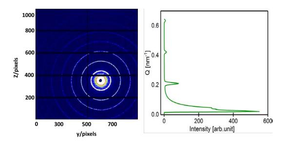
Figure 3.15.: AgBH calibration to determine the beam center and the sample-todetector distance. In the left, the measured intensity recorded on the detector. on the right, the transferred measured intensity to polar coordinates, where from the projection on Q, the optimal parameters for beam center and sample-to-detector distance are determined.
