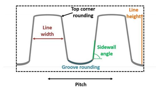
Figure 4.17.: A sketch of the grating model which explains and confirms the GISAXS data.
