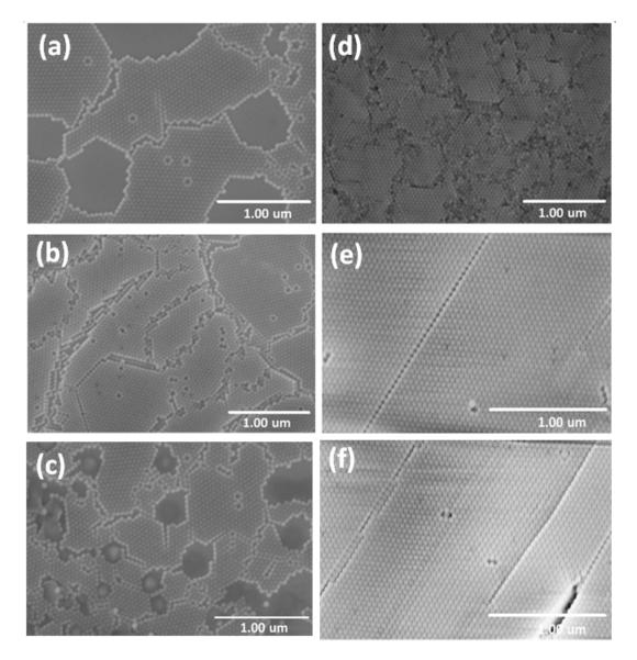
Figure 5.5.: SEM images of SiO<sub>2</sub> NPs with 0.11 vol% concentration (left) and SiO<sub>2</sub> NPs with 5.4vol% concentration (right). Different region of the same samples are shown in (a-c) and (d-f), respectively. For both concentrations, simple drop-casting method was used to deposit the nanoparticles in the wafer surface.
