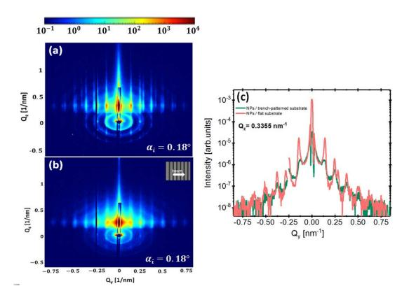
Figure 5.24.: Comparison between self-assembled particles in flat and trenchpatterned substrate. (a) GISAXS pattern of self-assembled stearyl silica particles monolayer on flat surface after 10 days in the oven with stearyl alcohol assistant. (b) GISAXS pattern of directed self-assembled stearyl silica particles on trench-patterned silicon substrate after 10 days in the oven with stearyl alcohol assistant. (c) Line-cut from (a) and (b) along  $Q_y$  at a fixed  $Q_z = 0.3355$  nm<sup>-1</sup>.
