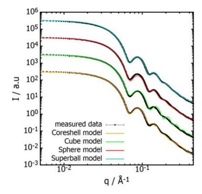
Figure 7.3.: The SAXS data of the iron oxide nanoparticles dispersed in toluene. Spherical (red), core-shell (yellow), cubic (violate) and superball (light blue) form factors were used to fit the data.
