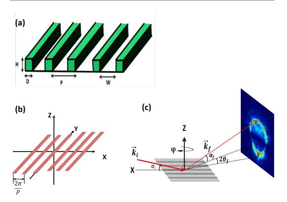
Figure 4.1.: Schematic representation of grating lines with period P, mesa width D, groove width W and height H. (a) Cross-sectional view in real space. (b) Reciprocal space representation of grating lines. (c) Scattering of a collimated X-ray beam from grating lines oriented parallel with respect to the incident beam (i.e.  $\phi = 0^{\circ}$ )
