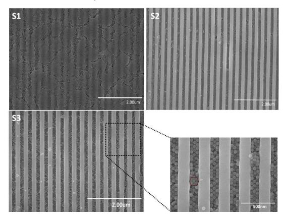
Figure 5.21.: SEM images of self-assembled silica nanoparticles of ≈ 50 nm diameter on the trench-patterned silicon substrate. (a) S1-sample, (b) S2-sample and (c) S3-sample, the inset is a magnified SEM image of a close-packed pattern indicated as the black rectangle in (c).
