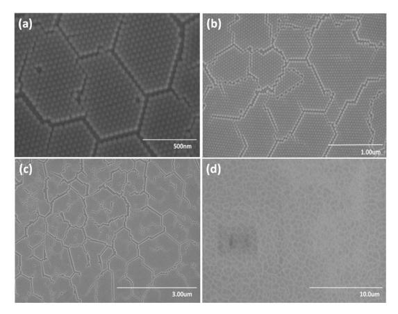
Figure 5.9.: Series of SEM images (a)-(d) with various magnifications, taken at different positions of a monolayer of SiO<sub>2</sub> NPs, assembled on a silicon wafer after using stearyl alcohol as assistant.
