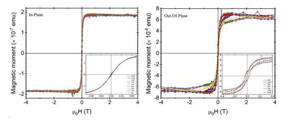
Figure F.3.: In-plane and out-of-plane hysteresis loops of the ordered  $CoFe_2O_4$  NP monolayers measured at various temperature. The downright insets is an expanded low-field curve.
