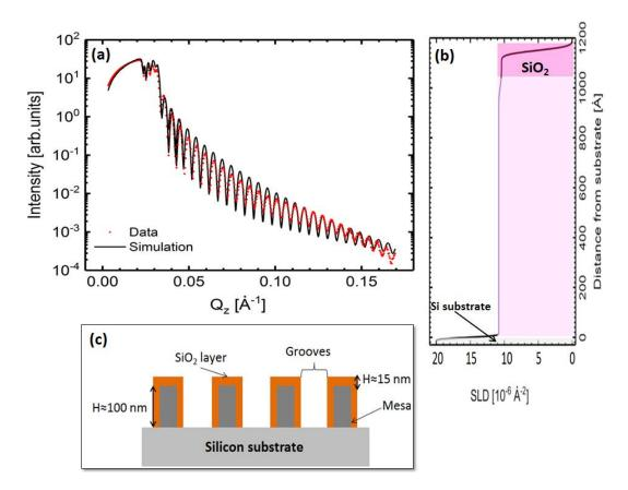
Figure 4.5.: (a) X-ray reflectivity as a function of momentum transfer (Q) of grating lines. Data shown as red symbols and fits shown as the black solid line. Parameters of the fit are displayed in table 4.1. (b) Modeled scattering length density (SLD) as a function of distance from air interface. (c) Sketch of the model used for fitting XRR data with the relevant parameters that are used to describe it.
