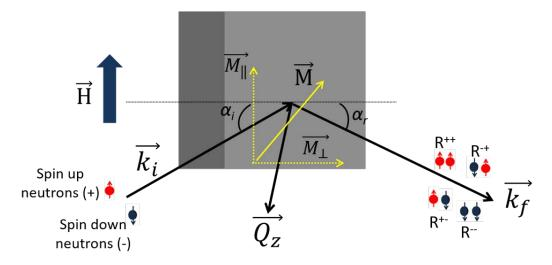
Figure 3.23.: Typical configuration of specular PNR experiment. Neutrons are polarized, either parallel or antiparallel to the external magnetic field  $\vec{H}$ . The  $\vec{M}_{\parallel}$  and  $\vec{M}_{\perp}$  are the two projections of M with respect to  $\vec{H}$ .
