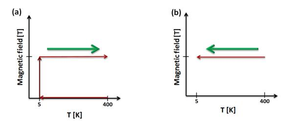
Figure 3.12.: Measurement procedures for (a) zero filed cooling and (b) filed cooling, where green arrows mark the paths along which the magnetization is recorded.
