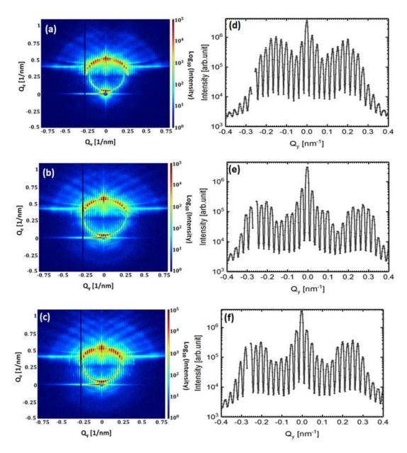
Figure 4.20.: GISAXS data at an incident angle  $\alpha_i=0.35^{\circ}$  for (a) S3\_01, (b) S3\_02 and (c) S3\_03. The bottom images displays the intensity as a function of  $Q_y$  along the semicircle for (d) S3\_01, (e) S3\_02 and (f) S3\_03.
