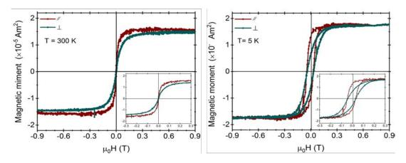
Figure 7.12.: Hysteresis loops for the cubic iron oxide nanoparticles on trenchpatterned silicon substrate measured at 300 K (left) and at 5 K (right). The brown hysteresis loops in both figures were measured as the filed parallel to the long axis of the trenches, the green ones were measured with the field perpendicular to the trenches.
