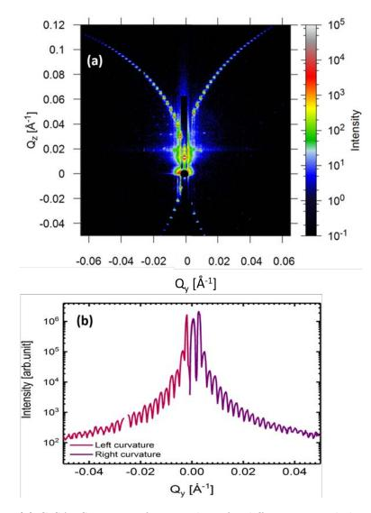
Figure 4.9.: (a) GISAXS pattern of grating lines for different azimuthal rotation close to the parallel orientation  $\phi = 0^{\circ}$  recorded at  $\alpha_i = 0.085^{\circ}$ . GISAXS pattern at right recorded at  $\phi = 6.3^{\circ}$  while at left recorded at  $\phi = 9.5^{\circ}$ . (b) The extracted average intensity profile  $I(Q_y)$  as a function of  $Q_y$ , where the violate line represents the right curvature and the pink line represents the left curvature.
