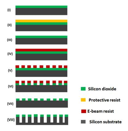
Figure 4.12.: Grating lines fabrication by e-beam lithography (EBL) method.
