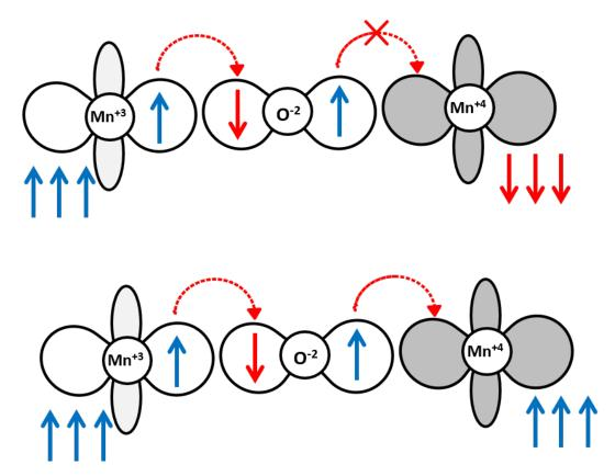
Figure 2.2.: Double exchange interaction between  $Mn^{+3}$  and  $Mn^{+4}$  mediated by an  $O^{-2}$  ion. Inspired from [29].
