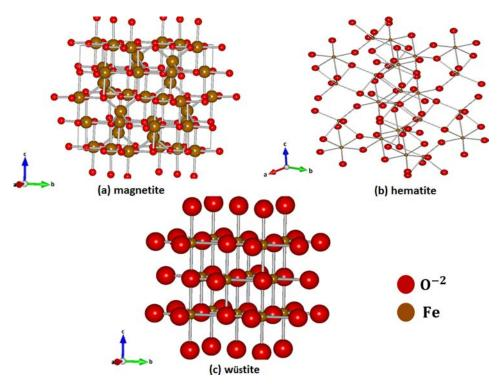
Figure 7.1.: Representation of iron oxide structure of (a) magnetite, (b) hematite and (c) wüstite. The red spheres represent the close-packed  $O^{2-}$  ion and the brown spheres indicate the position of the iron cations occupy either the tetrahedral or octahedral interstices. The visualization was produced using VESTA software [167] where the data used here are obtained from the Inorganic Crystal Structure Database (ICSD).
