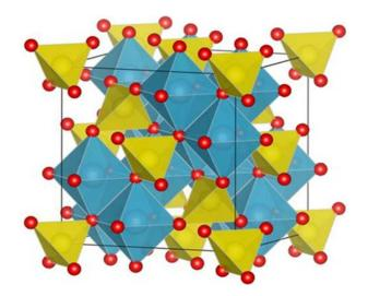
Figure 6.1.: Crystal structure of  $CoFe_2O_4$ . The Co atoms sit within the yellow tetrahedral and the Fe atoms sit within the blue octahedral. The red points represents the oxygen ions.
