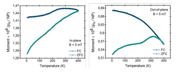
Figure 6.13.: Temperature dependence of the in-plane (left) and out-of-plane (right) magnetization of  $CoFe_2O_4$  nanodots on Si substrate at 50 mT. The blue and green curves are the field-cooling and zero-field-cooling curves, respectively.
