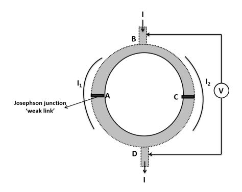
Figure 3.6.: Superconducting Quantum Interference Device (SQUID) as simple magnetometer.
