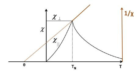
Figure 2.6.: Magnetic susceptibility vs.temperature for antiferromagnetic material.
