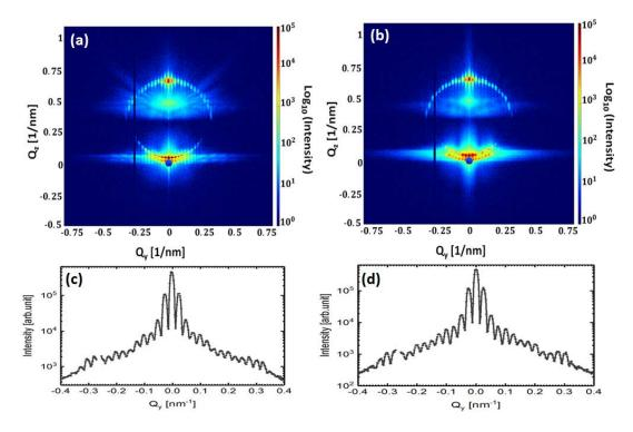
Figure 4.18.: GISAXS patterns at an incident angle  $\alpha_i=0.4^\circ$  for (a) S1\_01 and (b) S1\_02. The bottom right and left-hand images display the intensity as a function of  $Q_y$  along the semicircle for (d) S1\_01 and (e) S1\_02.
