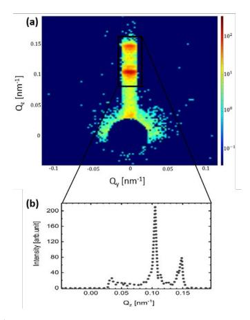
Figure 4.6.: (a) GISAXS scattering image of grating lines at  $\alpha_i = 0.06^{\circ}$  as the incoming beam perpendicular to the lines. (b) Intensity profile along the vertical specular axis as a function of  $Q_z$ . The peak position at 0.1  $nm^{-1}$  represents the specular peak.
