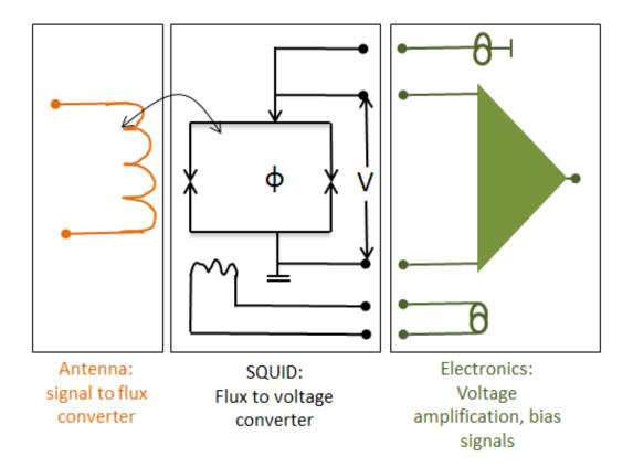
Figure 3.11.: SQUID = flux to voltage converter
