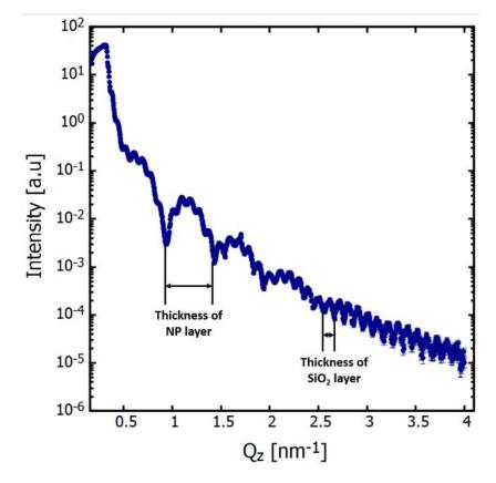
Figure 6.8.: X-ray reflectometry of the  $CoFe_2O_4$  monolayer prepared by a high temperature treatment.
