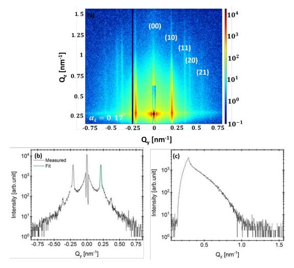
Figure 6.9.: (a) GISAXS pattern of CoFe<sub>2</sub>O<sub>4</sub> NPs grown on top of Si substrate at  $\alpha_i$ = 0.17°. The indexing of the Bragg rods according to a 2D hexagonal lattice with a = 34 nm is also shown. (b) A horizontal line cut of the GISAXS pattern at a fixed Q<sub>z</sub> = 0.29 nm<sup>-1</sup> along with Voigt fit (light green line) to (10) Bragg peak. (c) A vertical line cut of the GISAXS pattern at a fixed Q<sub>y</sub> = 0.21 nm<sup>-1</sup>.
