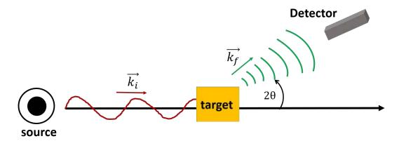
Figure 2.9.: Schematic of the general scattering process. An incoming wave with a wave vector  $k_i$  (red) interacts with the target (yellow) and produces an outgoing wave with wave vector  $k_f$  (green) then it is detected by a detector.
