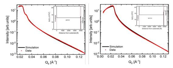
Figure 4.24.: X-ray reflectivity as a function of momentum transfer  $(Q_z)$  of (a) S1\_01 and (b) S1\_02 grating lines. Data shown as red symbols and fits shown as black solid line. Inset shows the scattering length density (SLD) profile as a function of distance from air interface.
