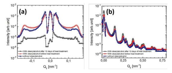
Figure 5.17.: Integrated intensity of the (a) diffuse rings and (b) Bragg rods as a function of  $Q_y$  determined from the GISAXS maps shown in figure 5.15 (a-c). The Bragg rods intensity is integrated from  $Q_z = 0.17 \text{ nm}^{-1} - 1.4 \text{ nm}^{-1}$  and the diffuse rings intensity is integrated from  $Q_z = -0.38 \text{ nm}^{-1} - 0.15 \text{ nm}^{-1}$ .
