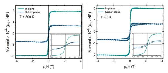
Figure 6.12.: In-plane and out-of-plane magnetization curves of  $CoFe_2O_4$  naodots on Si substrate at 300 K (left) and at 5 K (right).
