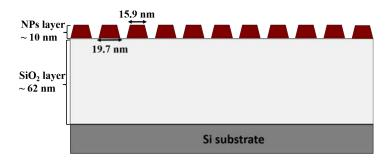
Figure 6.5.: A schematic drawing of the model assumed to fit the neutron reflectivity data. The sample can be modeled by a layered system of a silicon substrate (dark gray), silicon dioxide (light gray) and cobalt ferrite layer(brown). The hexagonal array layer of COF NP is modeled by a single slab of trapezoids.
