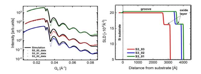
Figure 4.26.: Left side image : X-ray reflectivity as a function of momentum transfer  $(Q_z)$  of S3 grating lines. The data are shown as symbols and fits shown as a black solid line; red points correspond to S3\_03, blue points for S3\_02 and green points for S3\_01 points. The XRR curves for S3\_03 were multiplied by 10 and S3\_01 multiplied by 100. Right side image: SLD profiles as a function of distance from the air interface obtained by fitting XRR data in left side image.
