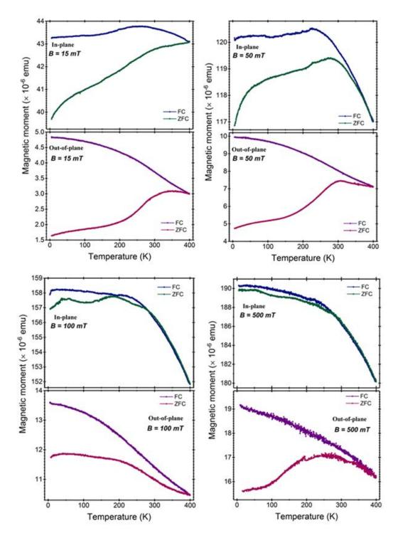
Figure F.2.: In-plane and out-of-plane temperature-dependent magnetization of the ordered  $CoFe_2O_4$  NP monolayers measured at various magnetic fields.
