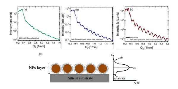
Figure 5.14.: X-ray reflectivity from a monolayer of  $SiO_2$  NPs (a) without stearyl alcohol. (b) with stearyl alcohol before heat treatment. ((c) with stearyl alcohol after 10 days of heat treatment (red points) along with the fit (black solid line). (d) The model layers structure assumed for fitting the data shown in (c), displaying an ideal in-plane close-packed arrangement of spherical nanoparticles with a parabolic SLD profile of the nanoparticles layer.
