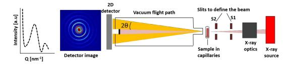
Figure 3.17.: Illustration of SAXS measurement principle, where the beam come from right to left.
