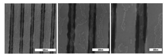
Figure 7.7.: SEM images from high to low magnification of self-assembled cubic iron oxide nanoparticles on the trench-patterned silicon substrate.
