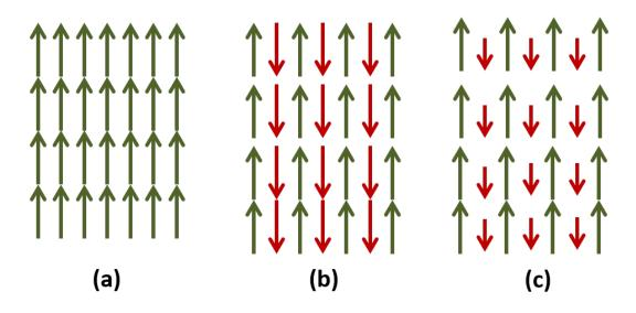
Figure 2.3.: Magnetic spin arrangements of (a) a ferromagnetism, (b) an antiferromagnetism and (c) a ferrimagnet.
