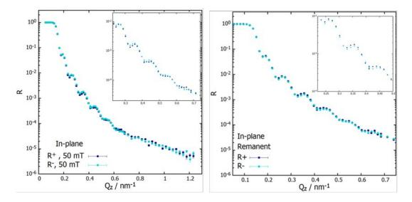
Figure F.4.: PNR measurements from COF nanodots onto a silicon substrate measured at 300 K with an applied In-plane field, (upper left) half polarized NR at 50 mT, (upper right) half polarized NR at remnant field.
