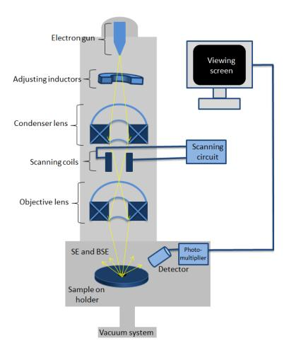
Figure 3.4.: Schematical setup for a scanning electron microscope.
