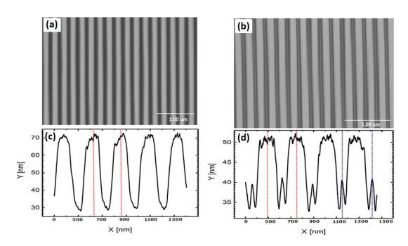
Figure 4.14.: (a) SEM image for S2\_01, (b) SEM image for S2\_02, (c) Line profile for S2\_01 and (d) Line profile for S2\_02.
