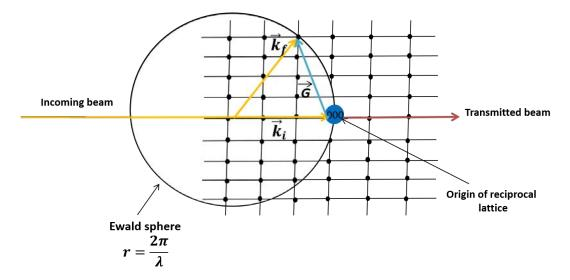
Figure 2.12.: Ewald sphere construction: When the reciprocal lattice point intersecting the sphere, the Bragg condition is satisfied.
