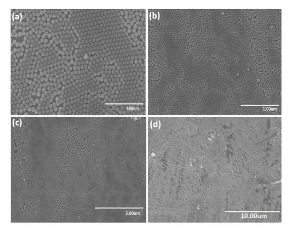
Figure 5.8.: Series of SEM images (a)-(d) with various magnifications, taken at different positions of a monolayer of SiO<sub>2</sub> NPs, assembled on a silicon wafer with extra toluene added after drop casting (without stearyl alcohol).
