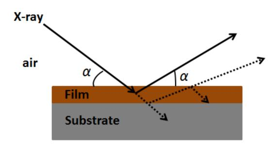
Figure 3.20.: Schematic of X-ray reflectometry measurement.
