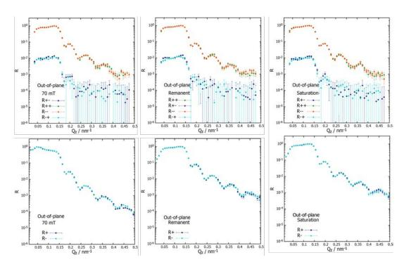
Figure F.5.: PNR measurements from COF nanodots onto a silicon substrate measured at 300 K with an applied Out-of-plane field. The upper plots show a full polarized NR measured at 70 mT, remnant and saturation, respectively. The bottom plots show a half polarized NR measured at 70 mT, remnant and saturation, respectively.
