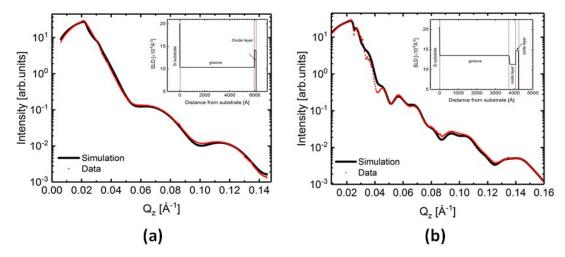
Figure 4.25.: X-ray reflectivity as a function of momentum transfer  $(Q_z)$  of (a) S2\_01 and (b) S2\_02 grating lines. Data shown as red symbols and fits shown as the black solid line. Inset shows the scattering length density (SLD) profile as a function of distance from air interface.
