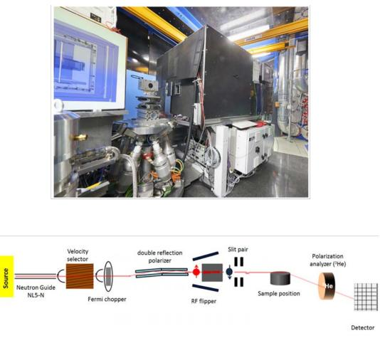
Figure 3.21.: The MARIA instrument at Heinz Maier-Leibnitz Zentrum used for (polarized) neutron reflectometry.
