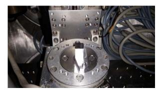
Figure 3.18.: The sample holder for the GISAXS experiment that can be tilted and moved in three dimensions.
