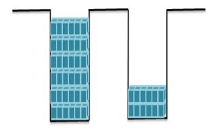
Figure 7.6.: Schematic drawing of the cubic nanoparticles inside trenches.
