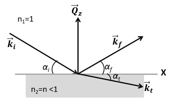
Figure 2.14.: Reflection and refraction from a surface.
