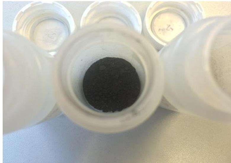
Figure 12. Polycrystalline Sample of the Mn<sub>5-x</sub>Fe<sub>x</sub>Si<sub>3</sub> Series produced by cold crucible melting after the grinding process.
