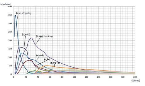
Fig. 1. Energy dependence of the cross sections of different neutron emitting reactions for deuterons impinging on Be.
