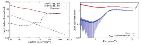
Fig. 11. Left: Scattering cross-sections for liquid ortho- $H_2$  (upper curve) and liquid para- $H_2$  (lower curve) from ENDF-VII. The para- $H_2$  is contaminated with a 0.5% admixture of ortho- $H_2$ . Right: Total cross section (including scattering and absorption) and scattering cross section of pure para- $H_2$ .
