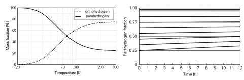
Fig. 13. Temperature-dependent thermodynamic equilibrium of ortho- to para-hydrogen mixtures (left) and change of hydrogen composition due to auto conversion over 12 hours in liquid hydrogen at 17 K and 0.15 MPa (right).
