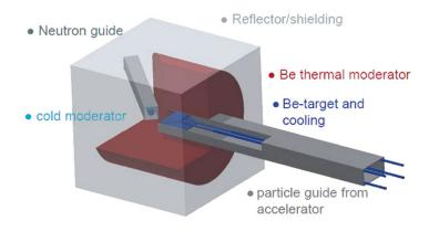
Fig. 6. Schematic drawing of a compact target-moderator setup with thermal and cold moderator.
