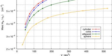
Fig. 7. Maximum thermal flux normalized to the number of primary neutrons depending on the volume of spherical, cylindrical, conical and elliptical beryllium moderators. The axes of symmetry of the moderator geometries and the beam direction of the source particles point in the positive z-direction. Since the volume of the latter three depends on two parameters, only the optimal parameter combination for a given volume is plotted.
