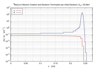
Fig. 5. Depth dependence of neutron production and  $D^+$  ion stopping probability for a 25 MeV deuteron beam on a bulk Be target. 99% of primary neutrons are produced up to a penetration depth of 0.225 cm while 0.2% of deuterons are deposited.
