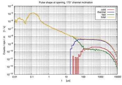
Fig. 10. Pulse shape of neutrons leaving the moderator at the channel opening. Neutrons with energy below 13.1 meV (150 K) are referred to as cold neutrons, below 127 meV (1474 K) as thermal neutrons and above as fast neutrons.
