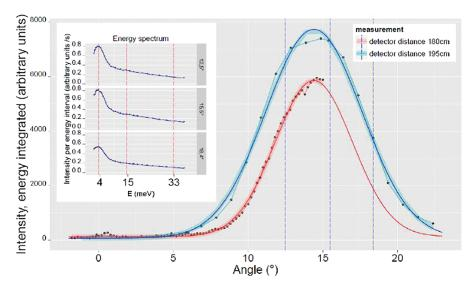
Fig. 9. Extracted thermal neutron beam of the  $D_2O$  moderator prototype at different detector distances at the TREFF beamline of MLZ.
