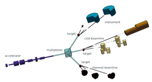
Fig. 16. Schematic layout of a future accelerator-driven high-brilliance neutron source.
