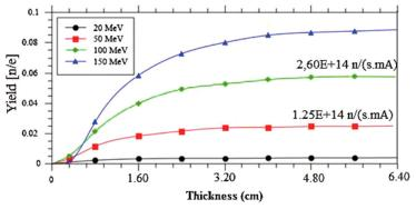
Fig. 4. Simulation of the neutron yield (per incident particle) for a uranium target for different electron energies as a function of target length.
