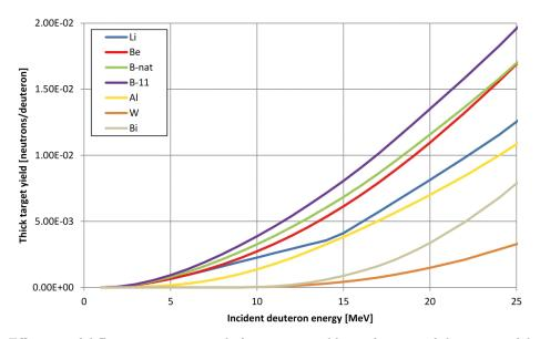
Fig. 2. Efficiency of different target materials for neutron yield as a function of the energy of deuterons.
