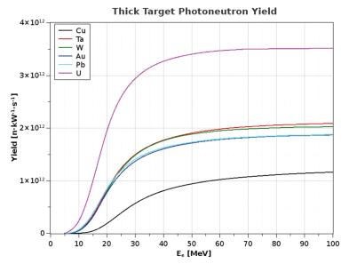
Fig. 3. Neutron yield (per kW power of an electron accelerator) for different materials for an electron beam as a function of the electron energy.
